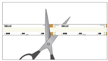
2 Cut the COB RGB strip to the required length by following the cutting mark, ensuring that you prevent damage to the light.
