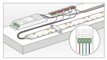
5 Connect the RGB controller to RGB strips to operating RGB functions. WAGO connectors enable quick wiring of LEDs in series. \*Polarity must be matched (+, -).
