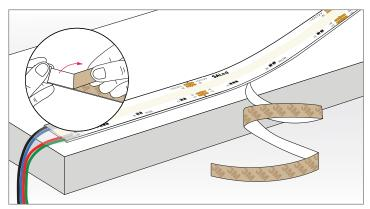
**3** Remove the adhesive tape, position the COB RGB strips carefully, ensuring they are straight, and press firmly. Avoid removing and reapplying the strip (see Figure 1 on page 2).
