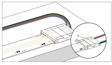
4 Our COB RGB Strip Connector enables quick, solder-free joining of wires or LED strips. Various connector types are available to suit specific applications (see Figure 2, page 2).
