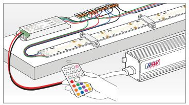
**6** Wire both ends of RGB strips to the power supply. For multiple series, connect them in parallel (refer to Figure 3 on page 2). Adjust the RGB strip with a remote control.
